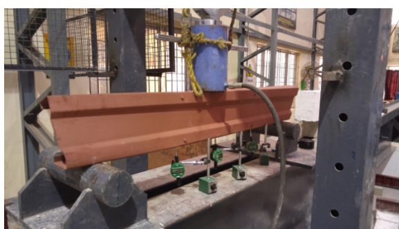
fig 4.10: flexure-torsional buckling failure (type 3)
